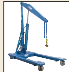
Ruger Adjustable Straddle Legs Fully Closed
