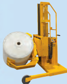
HER80060RCR2336-16 ER Roll Manipulator with RCR Clamp for 23" to 36" diameter rolls
