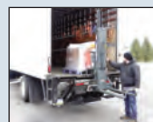
Release the pin and pull out bottom forks.
